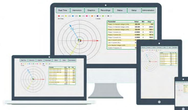
*The Web server graphic interface is the same displayed on the instrument touch screen. Both the instrument and the interface are multilingual.*
